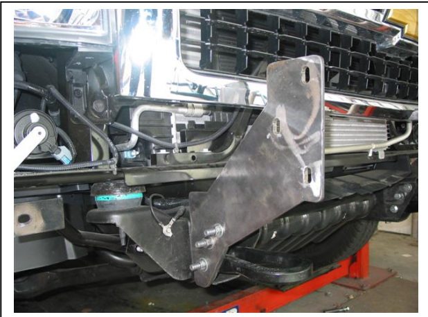
Figure 3: Drivers side steel mounting bracket fitted
