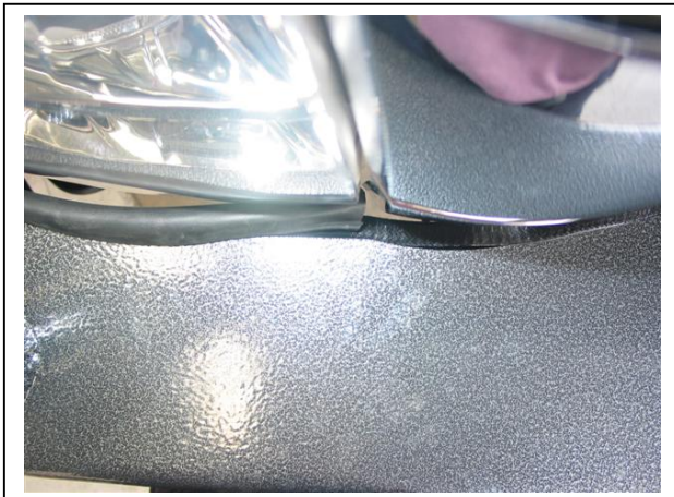
Figure 5a: infill trim cut point on bumper, fitted in picture.
